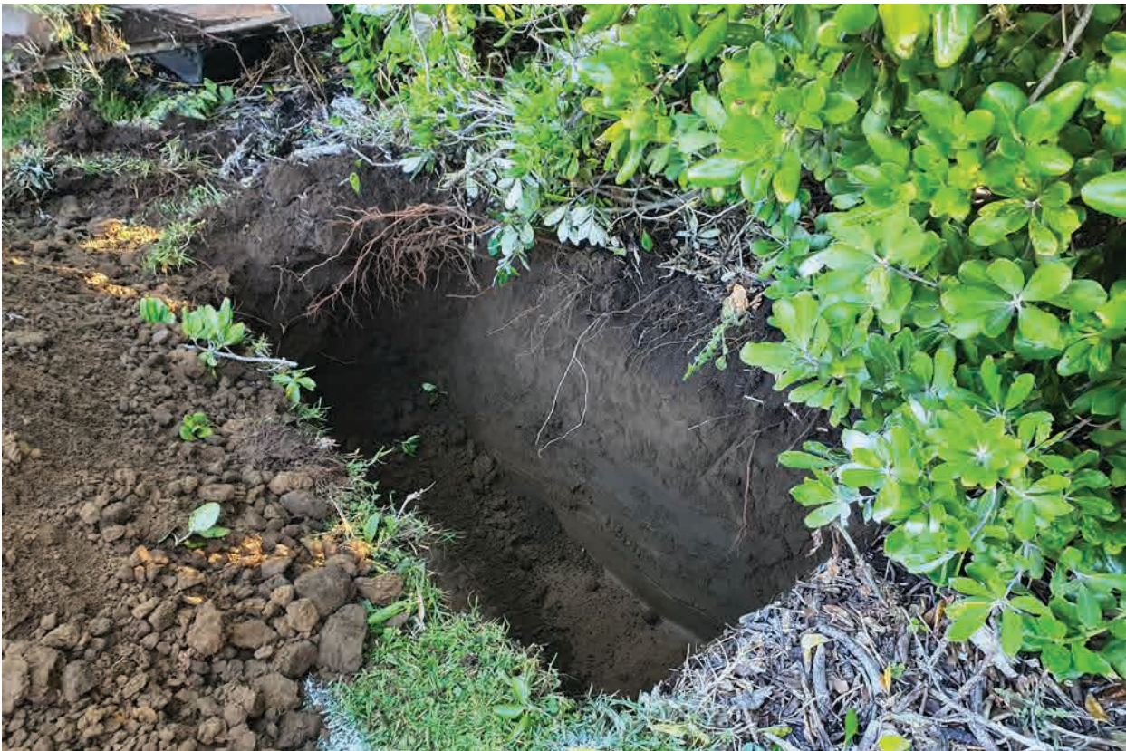
Figure 3. Insertion hole on Aria Terrace showing Egmont black soils. Depth of pit is 600 mm.
